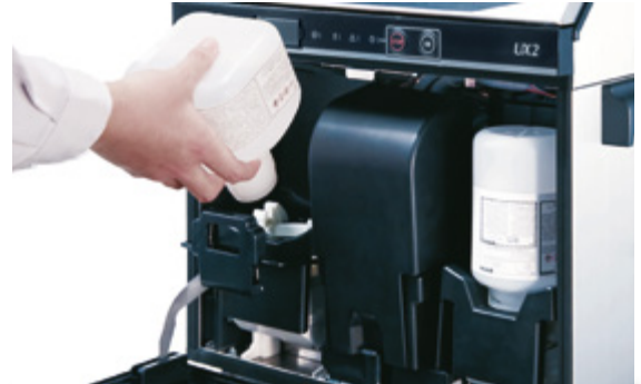
RFID prevents the installation of the wrong cartridge
